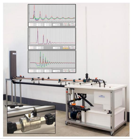
This equipment is used to visualize and study the phenomenon of water hammer.
