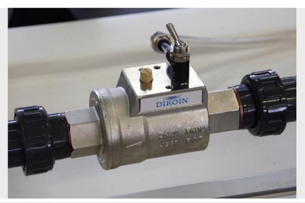
Optional Accessory: FL 09.1.VX - QUICK-CLOSING VALVE FOR WATER HAMMER The quick-closing valve, powered by compressed air, causes an almost instantaneous stop of the water circulation, thus generating the maximum possible water hammer in the line in which it is placed. NOTE: Requires compressed air line.
